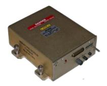
This precision high voltage power supply provides all operating voltages required for high resolution color displays. It provides a fixed 25kv anode voltage at up to 1200 microamperes with .05 percent regulation and only 2 volts of ripple.
