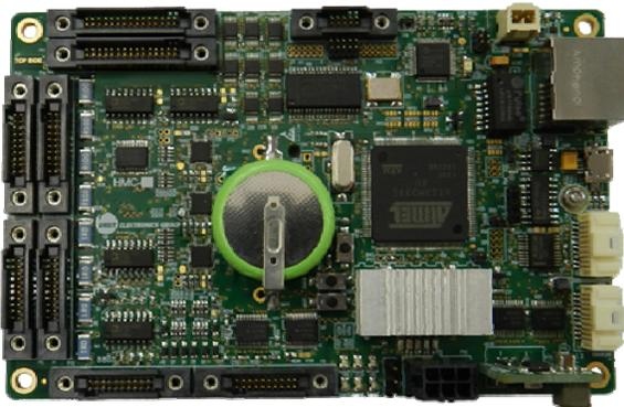
The Behlman IQCM Intelligent Chassis Manager is a stand-off mounted system manager that is compatible with ANSI/VITA 1.0 - VME64; ANSI/VITA 1.1 - VME64X; ANSI/VITA 46 - VPX; and ANSI/VITA 65 - OPEN VPX chassis. It supports VPX, VME and many other types of chassis.
